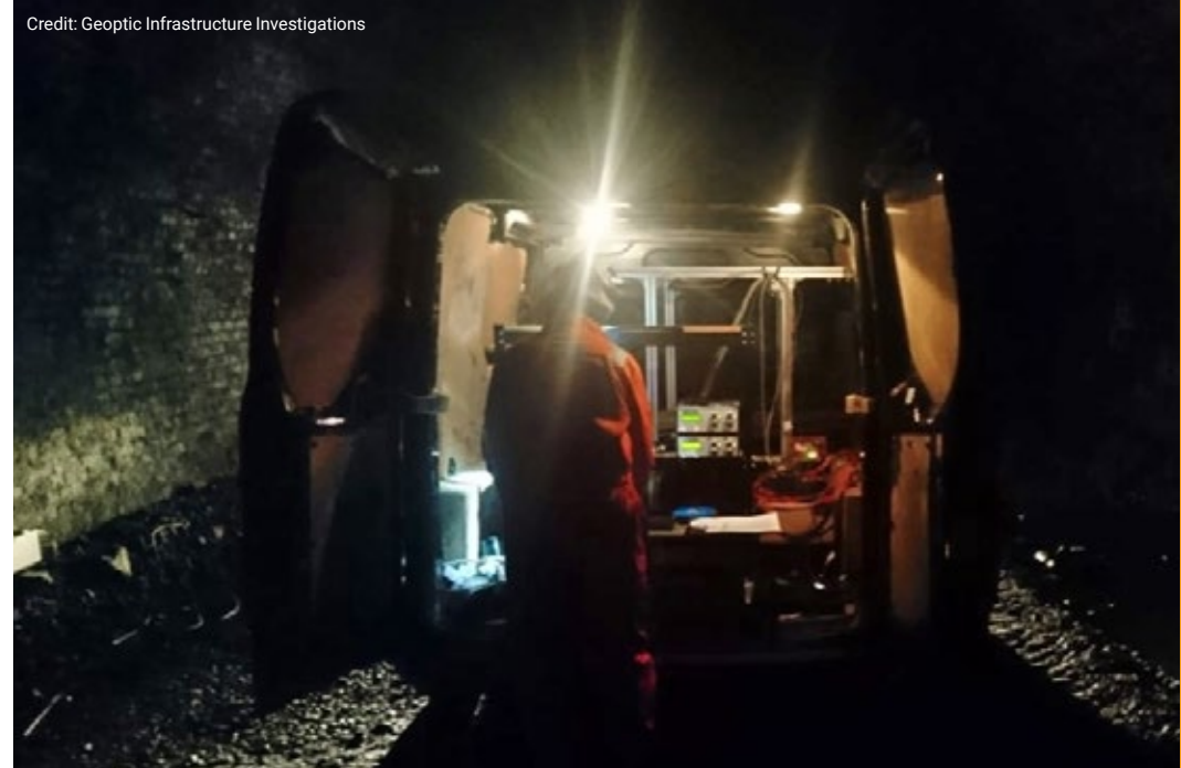
Muon tomography instrumentation imagining a railway tunnel
