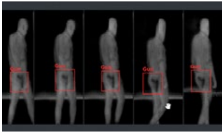
Left: Demonstration of our system working at Cardiff airport working at 5 frames/s. Here a mock gun has been concealed underneath a thick jacket. The system can clearly image the gun which has been identified by the AI as a threat. Centre: A CAD model of the early prototype demonstration system. Right: The demonstration system on temporary deployment at Cardiff airport.
